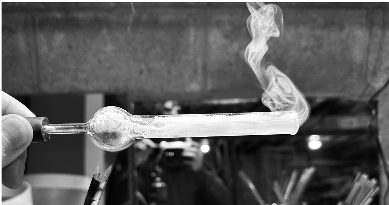
Fig. X.—Flame applied to the bulb while holding the device by the rubber stopper. The aquarium pump is connected to the rubber stopper and blowing air. Hold the specimen under the smoke or bring the device to the sample after heating. Heating the large stem (right) may help, as the smoke must be at a specific temperature for application to the surface.
