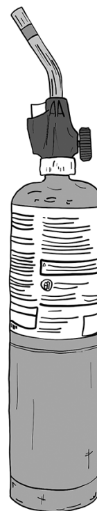
Fig. X.—Materials used to achieve a coating of ammonium chloride crystals on a fossil specimen. A , glass drying tube, rubber stopper, aquarium tubing, and an aquarium pump. B , propane cylinder and screw-on propane torch head.
